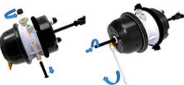
3. Turn on the parking brake on the vehicle. This is to exhaust all the air from inside of the spring brake.
