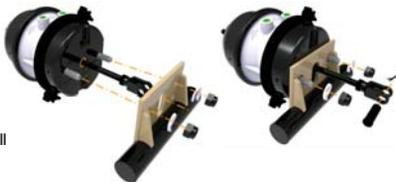
5. Make sure the location of the yoke nut and yoke at the pushrod, position the yoke hole to slack adjuster and make sure the external diameter of the yoke pin and assemble the split pin. Hold yoke to prevent it from turning and tighten yoke nut to 6~7kgf.m (45~50 lbf.ft) torque
